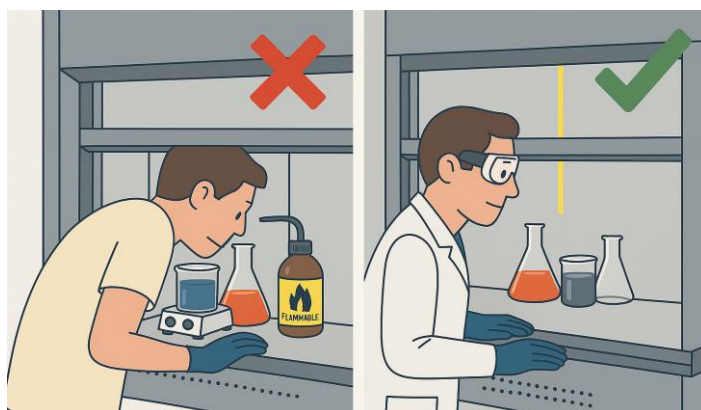
Figure 19: Incorrect and correct use of fume hoods
